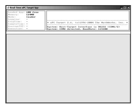
The xPC TargetBox and the loaded xPC Target kernel are now ready to accept commands from the host computer through either the RS-232 or Ethernet connection.
