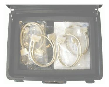
**Contents of the lower layer** — External I/O cables, xPC TargetBox User's Guide documentation, MPL hardware reference manual, and I/O reference manuals.
